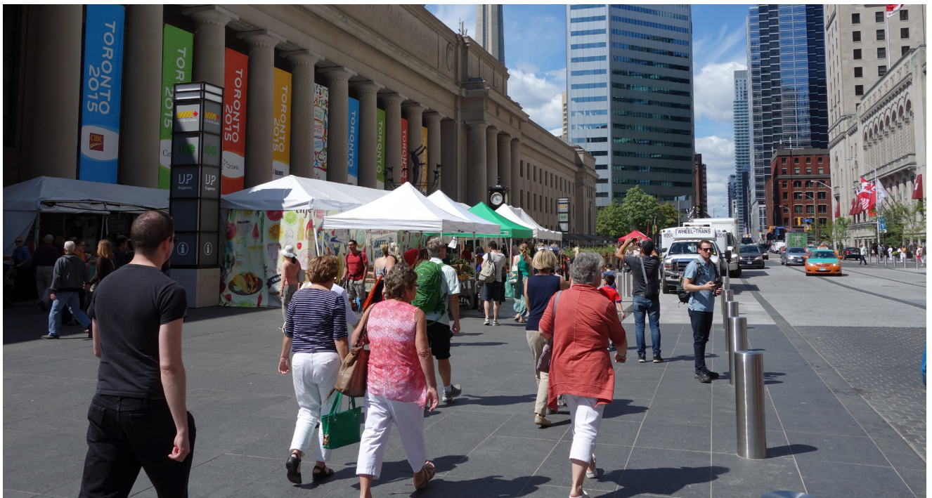
Plaza, bollards and roll and 'table-top' mid-block crossing in front of Union Station
