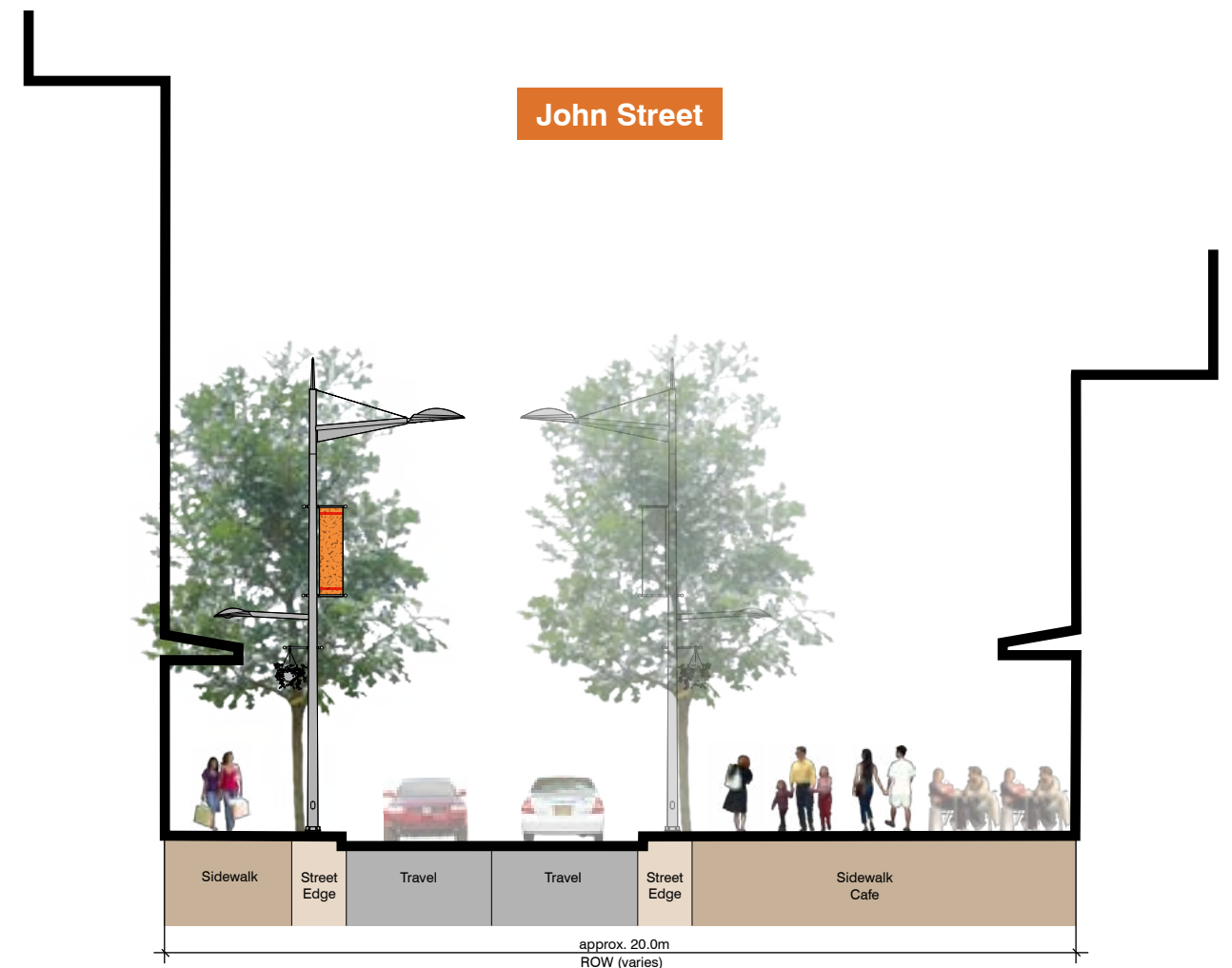
John Street Promenade Cross-section with two travel lanes and a wide promenade created on east side
